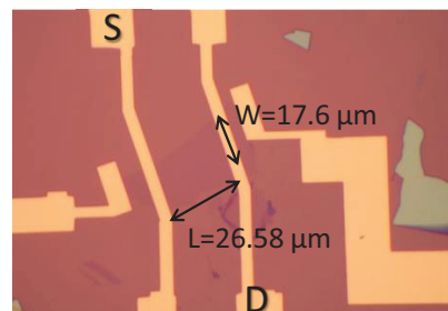
Fig. 1. Optical image of GFET S1 fabricated using mechanical exfoliation and electron beam lithography. The source (S) and drain (D) are as labeled.
