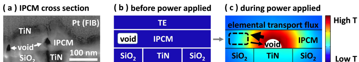
FIG. 4. (a) Cross-sectional SEM of an as-processed IPCM device prior to electrical probing, showing voids within the IPCM. (b) and (c) Conceptual diagrams illustrating possible J_{\text{RESET}} reduction mechanism: temperature gradients during RESET cause atomic diffusion from above the BE (hot region) to colder regions with voids (i.e., thermophoresis). Consequently, nearby voids are attracted above the BE, reducing the effective device size, thus reducing the apparent J_{\text{RESET}} .
